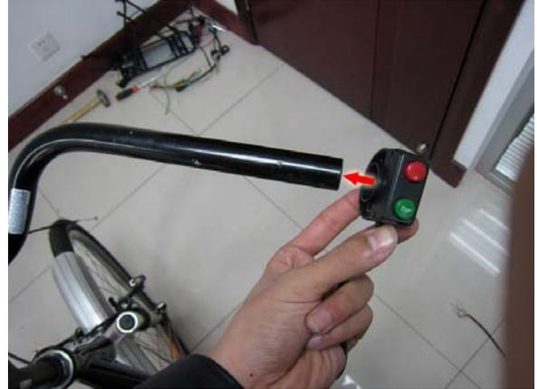
Place your hand on the handle bar and find the ideal position of the switch where your thumb is able to press the two buttons comfortably. Then use the 2.5mm Allen Wrench to tighten it.
