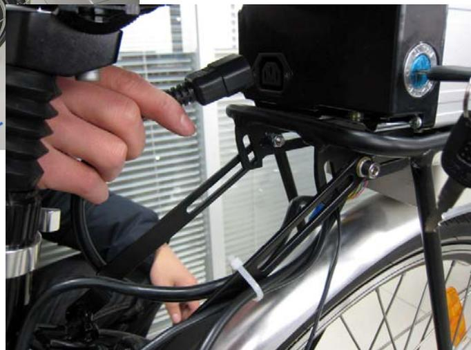
**Safety note:** Make sure the battery is turned off before you even plug in the power cable.
