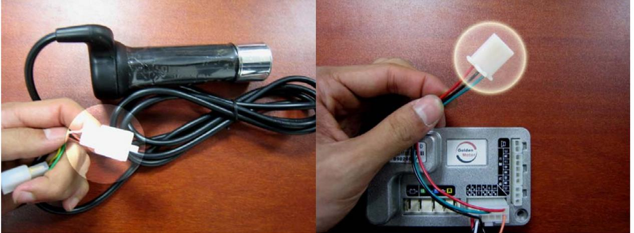
Take the throttle wire and single out the 3-hole pin connector.
