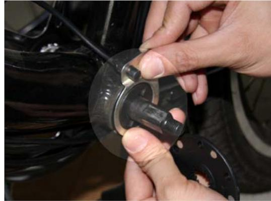
Place the outer magnetic ring next to the inner ring. Make sure they do not have any contact in between using washers.
