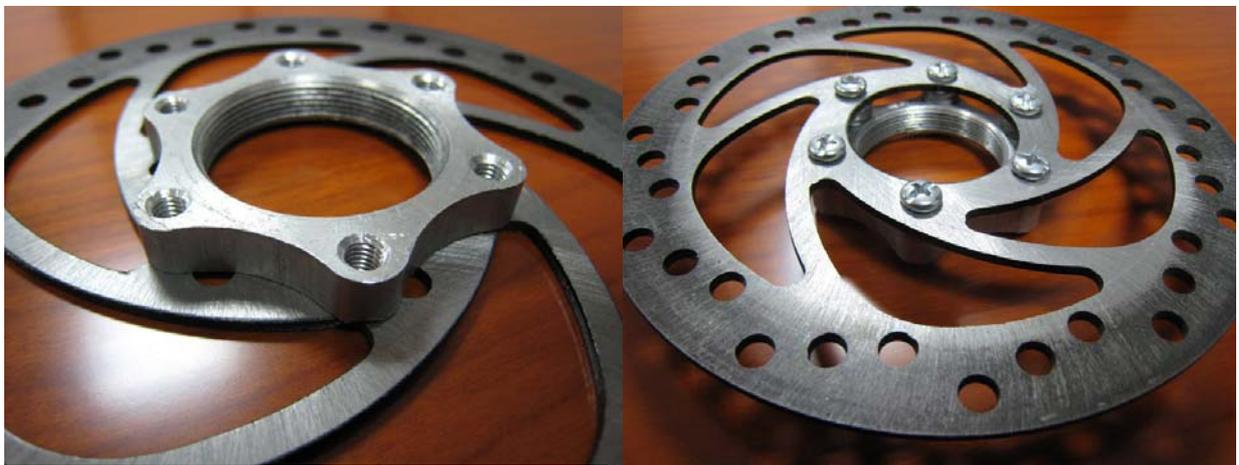
**Note:** Please confirm your Disc Brake diameter. (140mm or 160mm) In most cases, 140mm Disc Brakes are for the back wheel whilst 160mm are for the front wheel.
