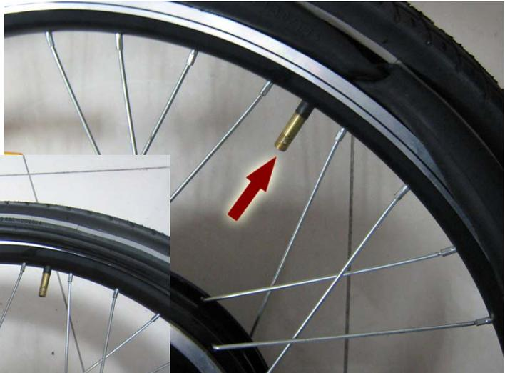
Stuff the rest of the inner tubing in between the rim and the outer tubing and you're done assembling the wheel!
