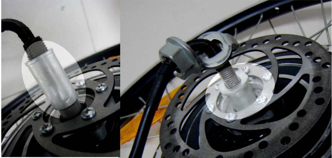
**Safety Note:** The Disc Brake Plate-Tube holds the disc brake in position. It is a very **important** component in the Disc Brake System.
