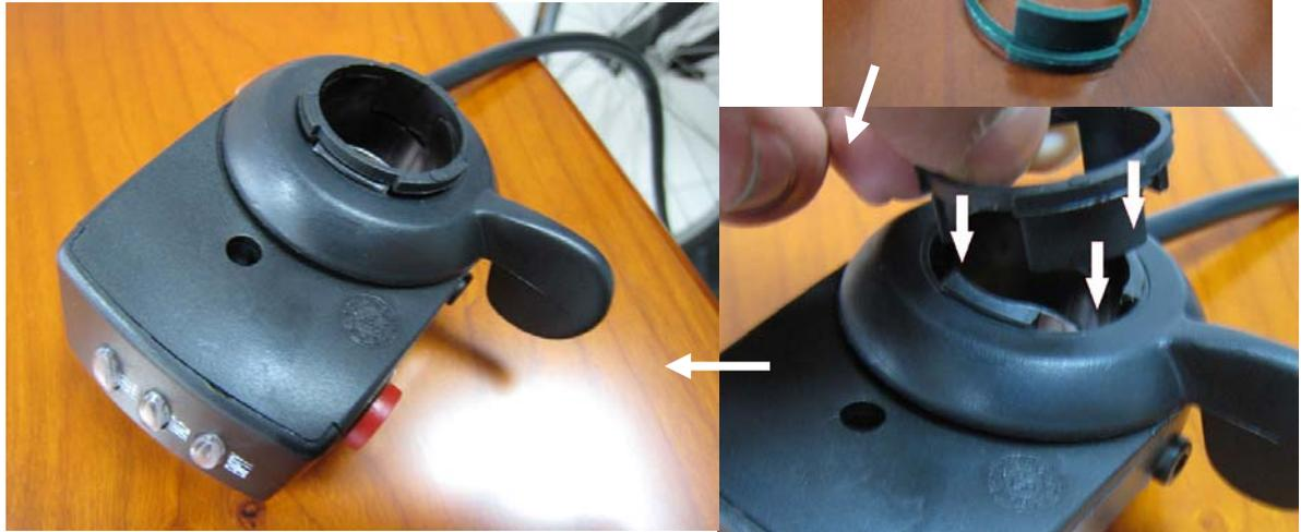
**Note:** This tripod comes useful if you are installing the thumb throttle on the right side of the steering bar. The tripod prevents the edge of the movable ring from getting stuck when it comes into contact with the exterior handle bars.
