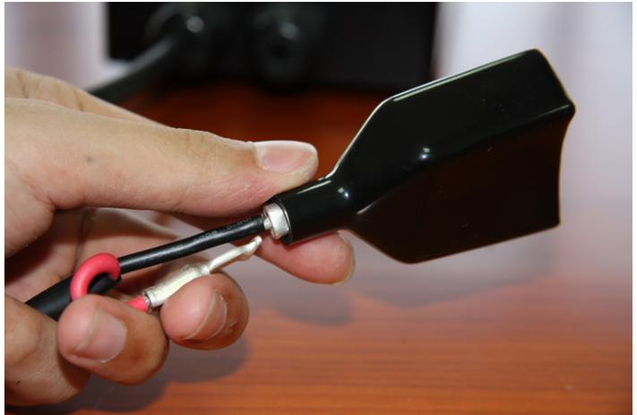
After the wire has been pushed through, push the bent wire in as well, this is because the neck of the protector is not big enough to fit both at the same time.
