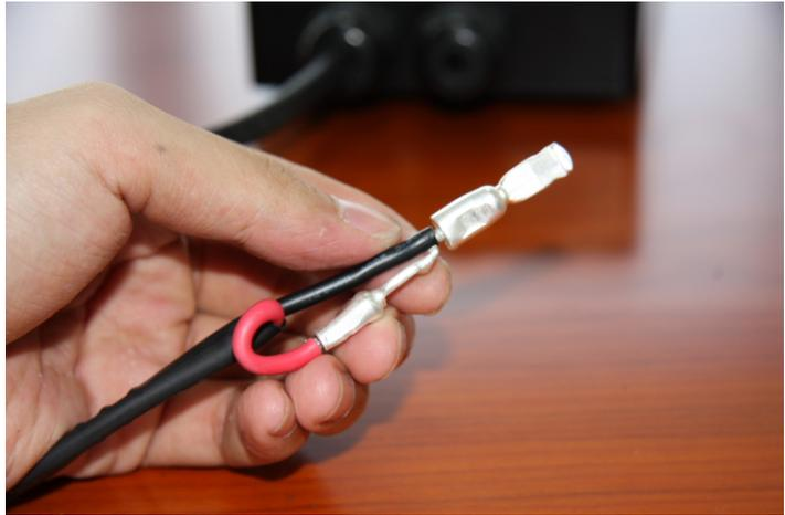
Slide in the unbent cable into the protector.
