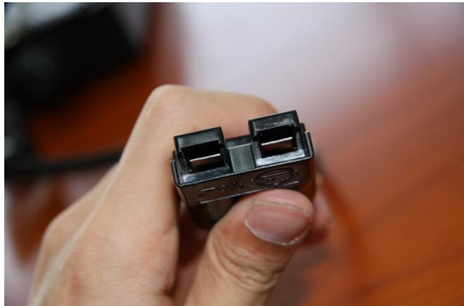
Make sure the “Nails of the Talon” has reached the end and clipped onto the metal plate. If this is done correctly, it is nearly impossible to pull out the power cord without tools.
